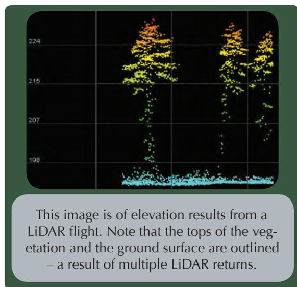
This image is of elevation results from a LiDAR flight. Note that the tops of the vegetation and the ground surface are outlined – a result of multiple LiDAR returns.
