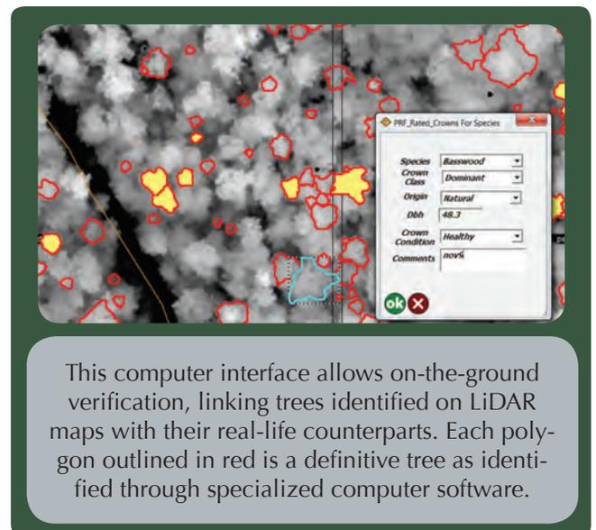
This computer interface allows on-the-ground verification, linking trees identified on LiDAR maps with their real-life counterparts. Each polygon outlined in red is a definitive tree as identified through specialized computer software.
